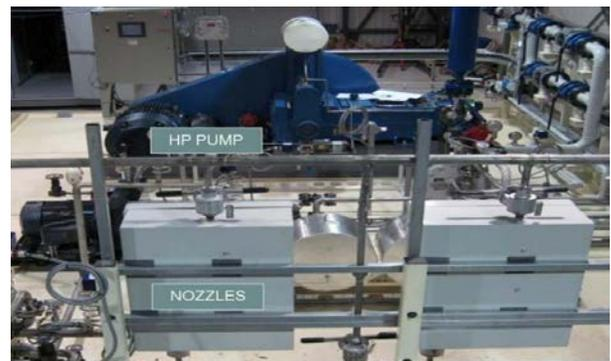
Figure 1 - JetShear nozzles and high-pressure pump
