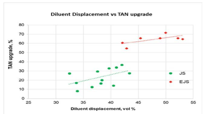
Figure 8 – Diluent Displacement vs TAN
