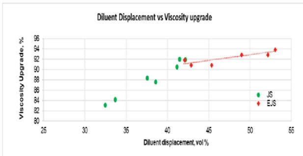
Figure 4 – Diluent Displacement vs Viscosity Upgrade
